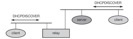
Figure Basic DHCP configuration
