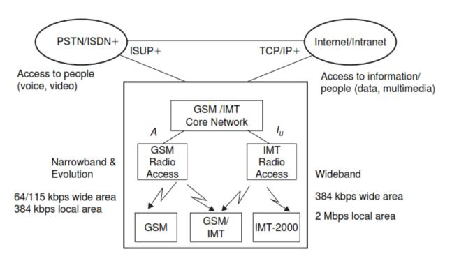
Figure 4.21 Evolution to UMTS/IMT-2000 in a GSM environment.
