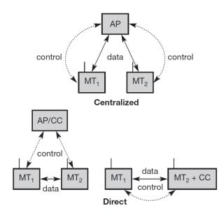
Figure 1.32 HiperLAN2 centralized vs direct mode
