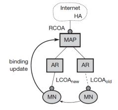
Fig: 2.12 Basic architecture of hierarchical mobile IP
