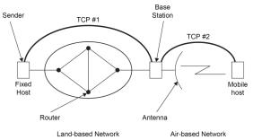
Figure Split connection (indirect) TCP in wireless environment.
