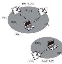
Station (STAi): terminal with access mechanisms to the wireless medium, Independent Basic Service Set (IBSS): group of stations using the same radio frequency
