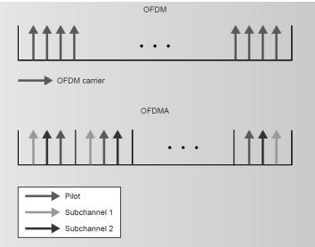
Figure 21.24 OFDM and OFDMA in 802.16e.
