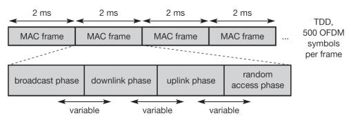
Figure 1.36 Basic structure of HiperLAN2 MAC frames
