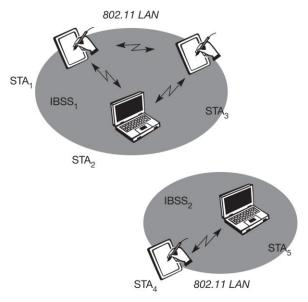
Figure 1.4 Architecture of IEEE 802.11 ad-hoc wireless LANs
