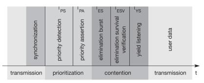
Figure: Phases of the HIPERLAN 1 EY-NPMA access scheme
