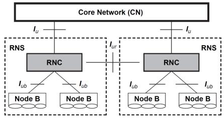
RNC: Radio Network Controller RNS: Radio Network Subsystem
