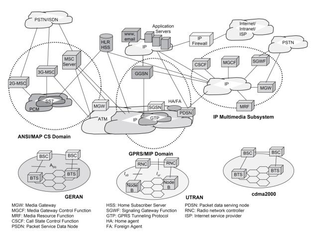
Figure 4.11 All-IP core network architecture for UMTS.
