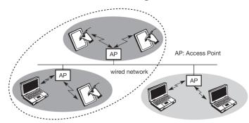
Figure: Example of three infrastructure-based wireless networks
