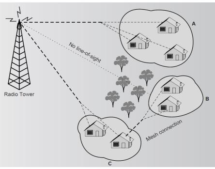
Figure 21.23 Mesh mode in IEEE 802.16 (WiMAX).
