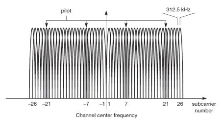
Figure 1.24 Usage of OFDM in IEEE 802.11a
