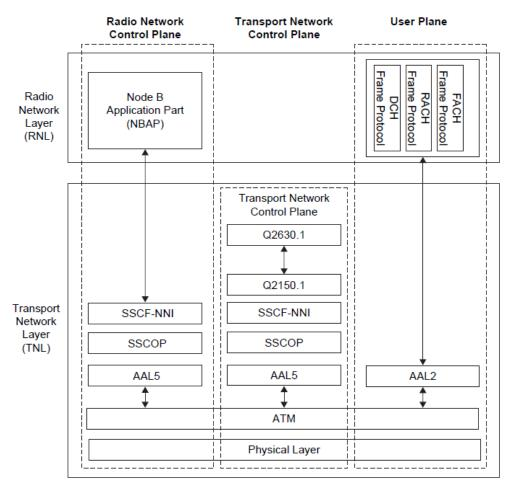
Figure 4.7 Protocol structure of *l*<sub>ub</sub> interface.
