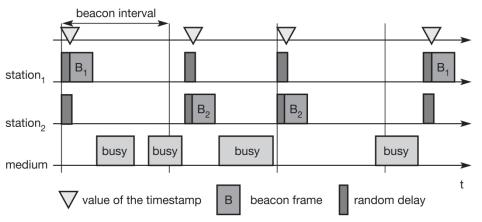
Figure: Beacon transmission in a busy 802.11 ad-hoc network
