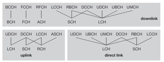
Figure 1.38 Mapping of logical and transport channels.
