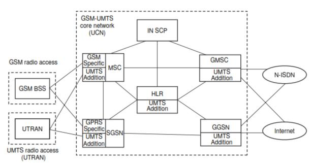
Figure 4.22 General GSM-UMTS network architecture.
