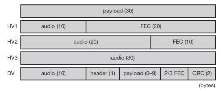
Figure 1.47 SCO payload types
