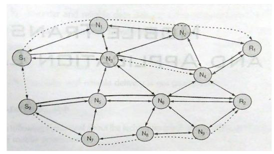
Figure: Example for Least Interference routing
