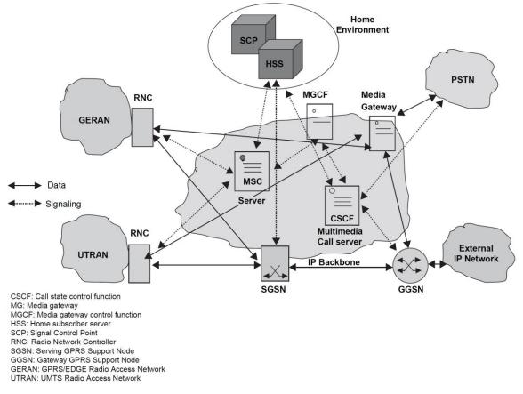
Figure 4.10 A simplified all-IP UMTS architecture.
