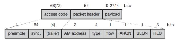
Figure 1.46 Baseband packet format
