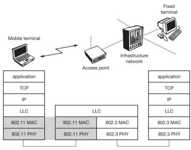
Figure: IEEE 802.11 protocol architecture and bridging
