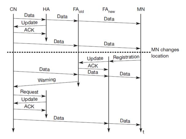
Fig 2.9 Change of the foreign agent with an optimized mobile IP
