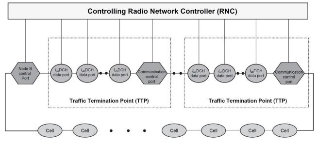
Figure 4.2 Node B logical architecture.
