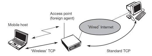
Figure 3.3 Indirect TCP segments a TCP connection into two parts
