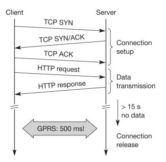
Figure 3.6 Example TCP connection setup overhead
