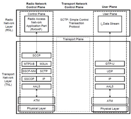
Figure 4.4 PS protocol architecture on lu interface.
