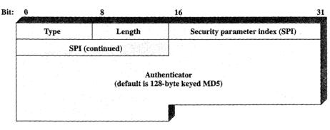
Figure 2.5 Mobile IP Authentication Extension
