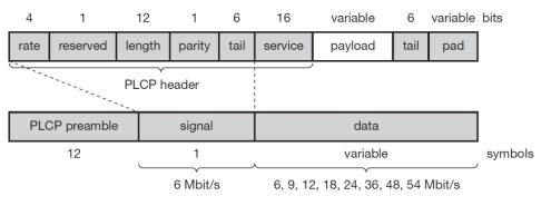
Figure 1.26 IEEE 802.11a physical layer PDU
