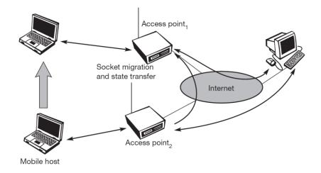
Figure 3.4 Socket and state migration after handover of a mobile host
