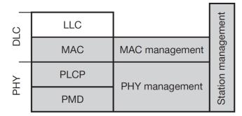
Figure 1.6 Detailed IEEE 802.11 protocol architecture and management
