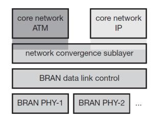
Figure 1.30 Layered model of BRAN wireless access networks
