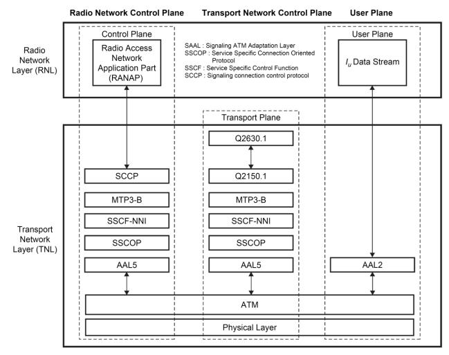
Figure 4.5 CS protocol architecture on lu interface.
