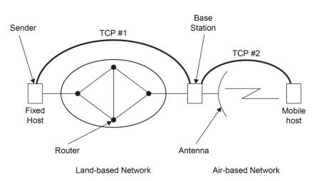
Figure 3.1 Split connection (indirect) TCP in wireless environment.
