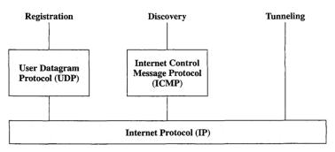
Figure 2.2 Protocol Support for Mobile IP
