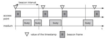
Figure: Beacon transmission in a busy 802.11 infrastructure network
