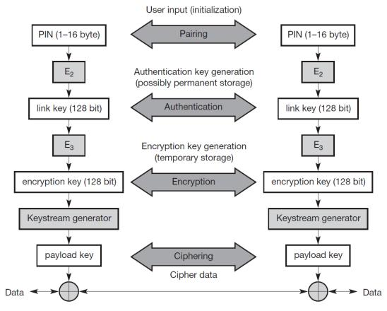
Figure 1.54 Bluetooth security components and protocols
