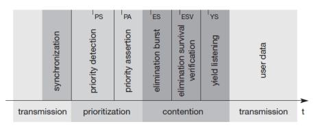
Figure 1.27 Phases of the HIPERLAN1 EY-NPMA access scheme
