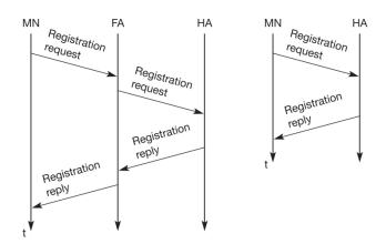
Figure: Registration of a mobile node via theFA or directly with the HA
