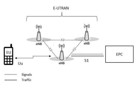
Figure 4.13: The E-UTRAN The access network
