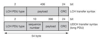
Figure 1.39 HiperLAN2 LCH and UDCH transfer syntax
