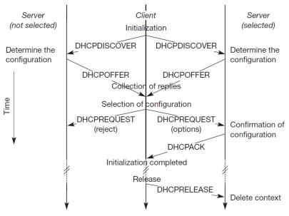
Figure Client initialization via DHCP
