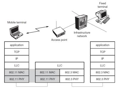
Figure 1.5 IEEE 802.11 protocol architecture and bridging
