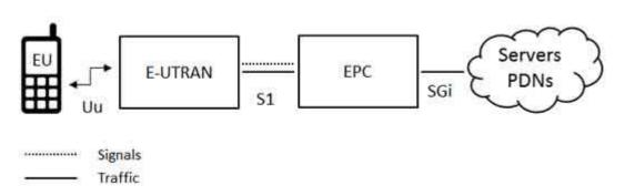
Figure 4.12 LTE network architecture
